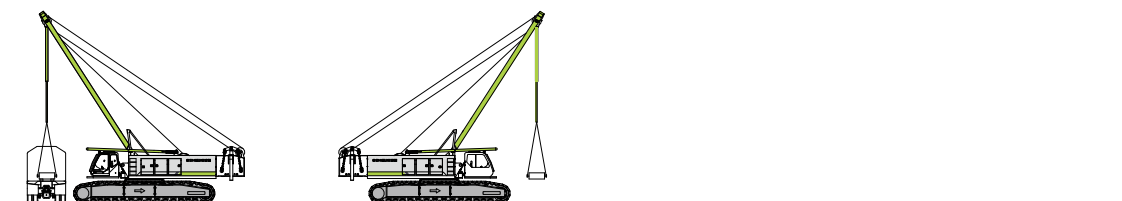
Unloading and assembly of central counterweight
