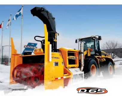
The D65 is a city snow blower with a ribbon conveyor; provides high performance for blowing snow windrows.
