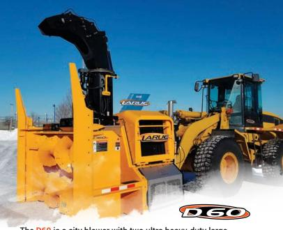
The D60 is a city blower with two ultra heavy-duty large screw conveyors; provides high performance in hard, icy snow conditions.
