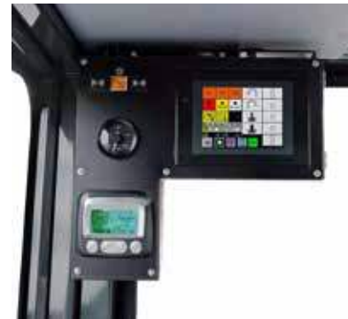
The monitoring system incorporates gauges in the cabin, allowing the operator a quick visual of engine temperature, hydraulic oil temperature and fluid levels.
