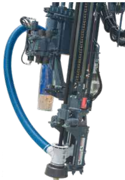
Sliding suction cup minimizes dust for better visibility.
